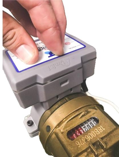
5. Place the supplied Cable cover over the pickup and Metrum cable entry and secure the cover with the provided screw and a small flat blade screwdriver.
