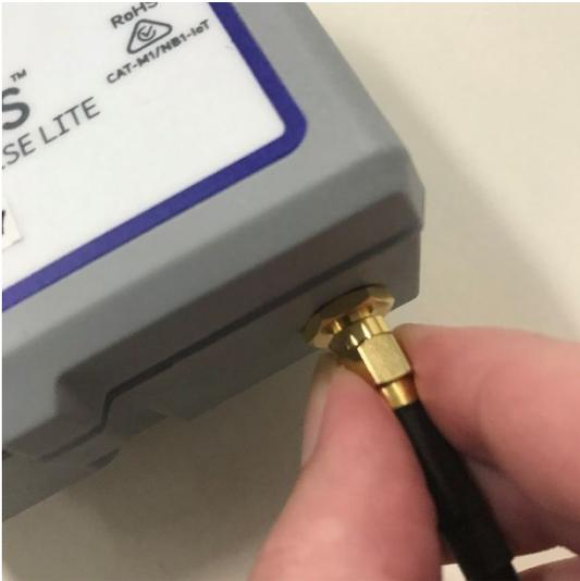
*Figure 3 External antenna connection*
